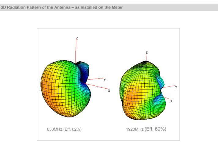
Note: The 3D Gain pattern and efficiency shown above is as measured with the antenna mounted on a particular GE meter at 3'O Clock position.
